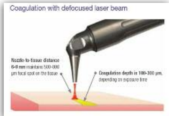
Figure 2. The difference between focused (a) and defocused (b) laser beams. Laser-tissue incision with focused (0.25 mm spot size) SuperPulse laser beam is illustrated. Defocused beam (> 1-2 mm spot size) with reduced fluence does not incise, but coagulates the tissue. Images are courtesy of LightScalpel, LLC, Bothell, WA.
