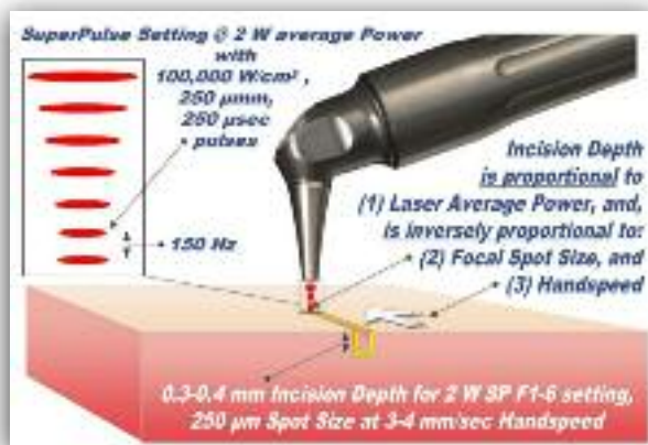
Figure 2. The difference between focused (a) and defocused (b) laser beams. Laser-tissue incision with focused (0.25 mm spot size) SuperPulse laser beam is illustrated. Defocused beam (> 1-2 mm spot size) with reduced fluence does not incise, but coagulates the tissue. Images are courtesy of LightScalpel, LLC, Bothell, WA.
